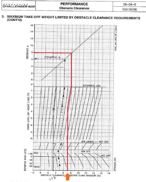
Obstacle Clearance Reference Climb Gradient, Flaps 20° – Anti-Icing Off (Page 2 of 2) Figure 06–04–3
