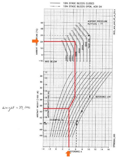
Obstacle Clearance Reference Climb Gradient, Flaps 20° – Anti-Icing Off (Page 1 of 2) Figure 06–04–3
