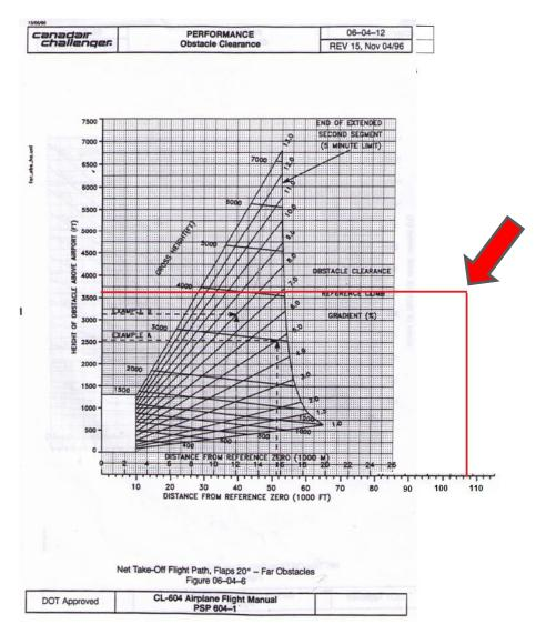
Note that the intersection of the red lines (red arrow above) is way to the right of the time limit line. The time it takes to reach the obstacle height at that climb rate far exceeds the 5 minute limit. This is <u>not</u> a viable option.
