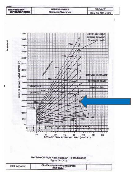
The second issue, that turning to this chart first would have revealed, is the engine time limit constraint. Note the right most vertical curved line of the chart (blue arrow above). This is the 5 minute limit line. In other words, an obstacle to the right of the line must be cleared significantly before reaching the obstacle. This is the case in this example.
