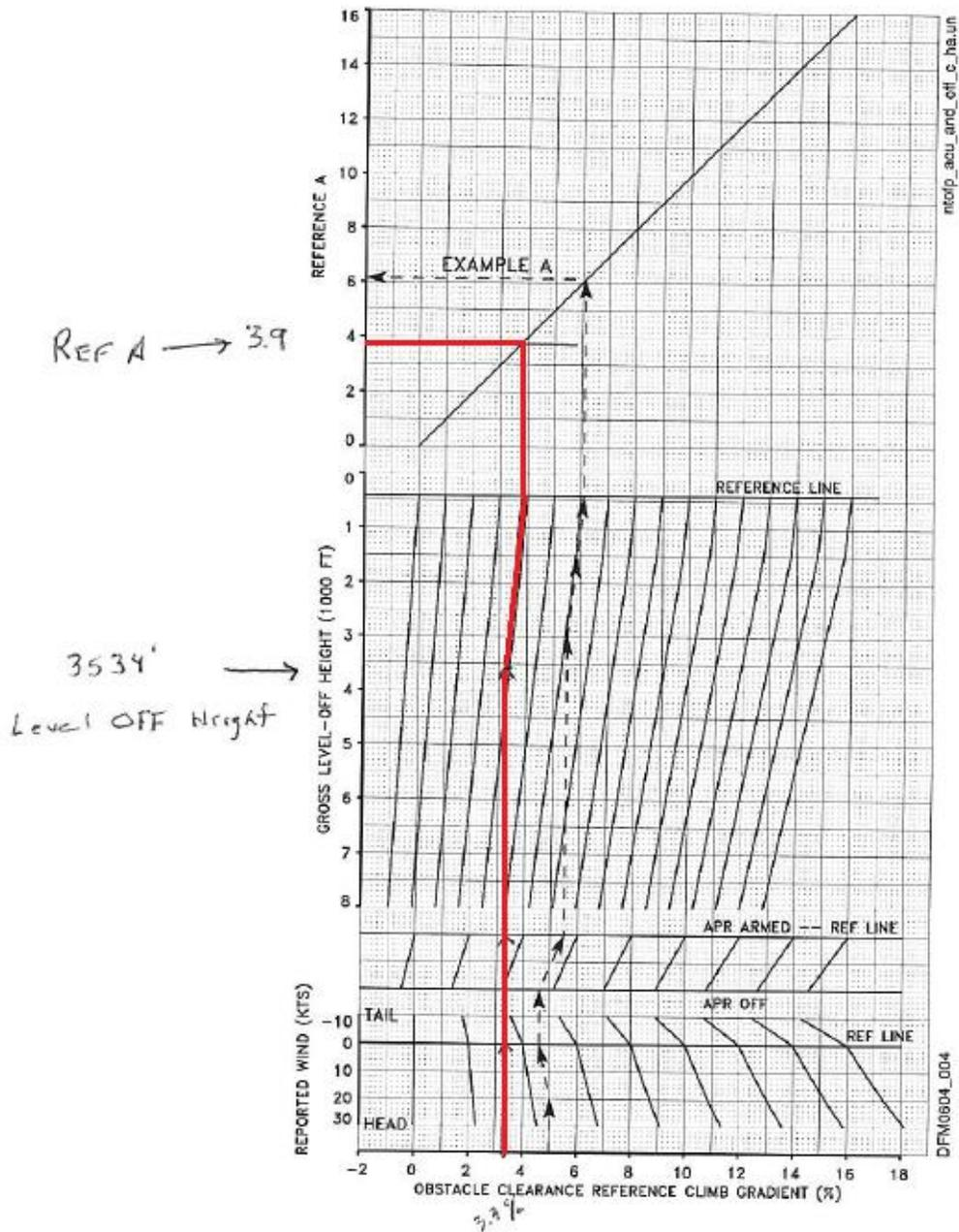
Obstacle Clearance Reference Climb Gradient, Flaps 20° - Anti-Icing Off (Page 2 of 2)
