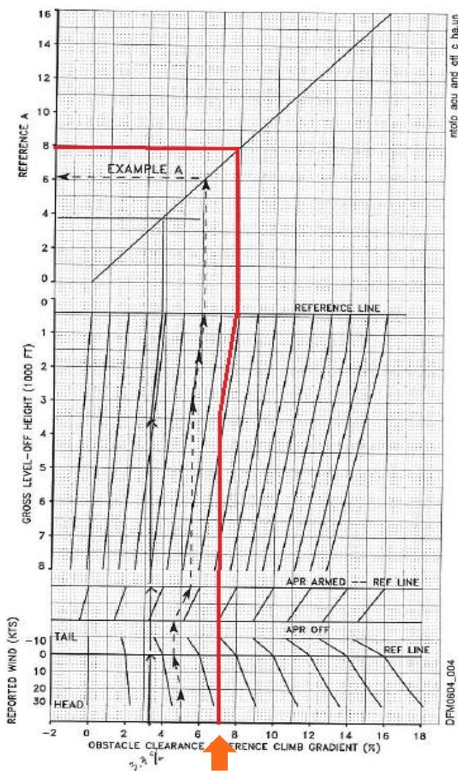
Obstacle Clearance Reference Climb Gradient, Flaps 20° – Anti-Icing Off (Page 2 of 2)
