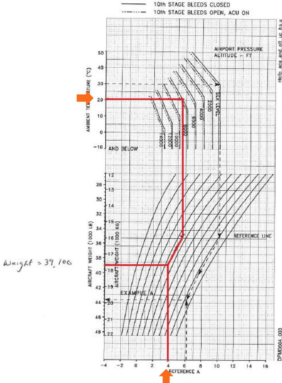
Obstacle Clearance Reference Climb Gradient, Flaps 20° - Anti-Icing Off (Page 1 of 2)
