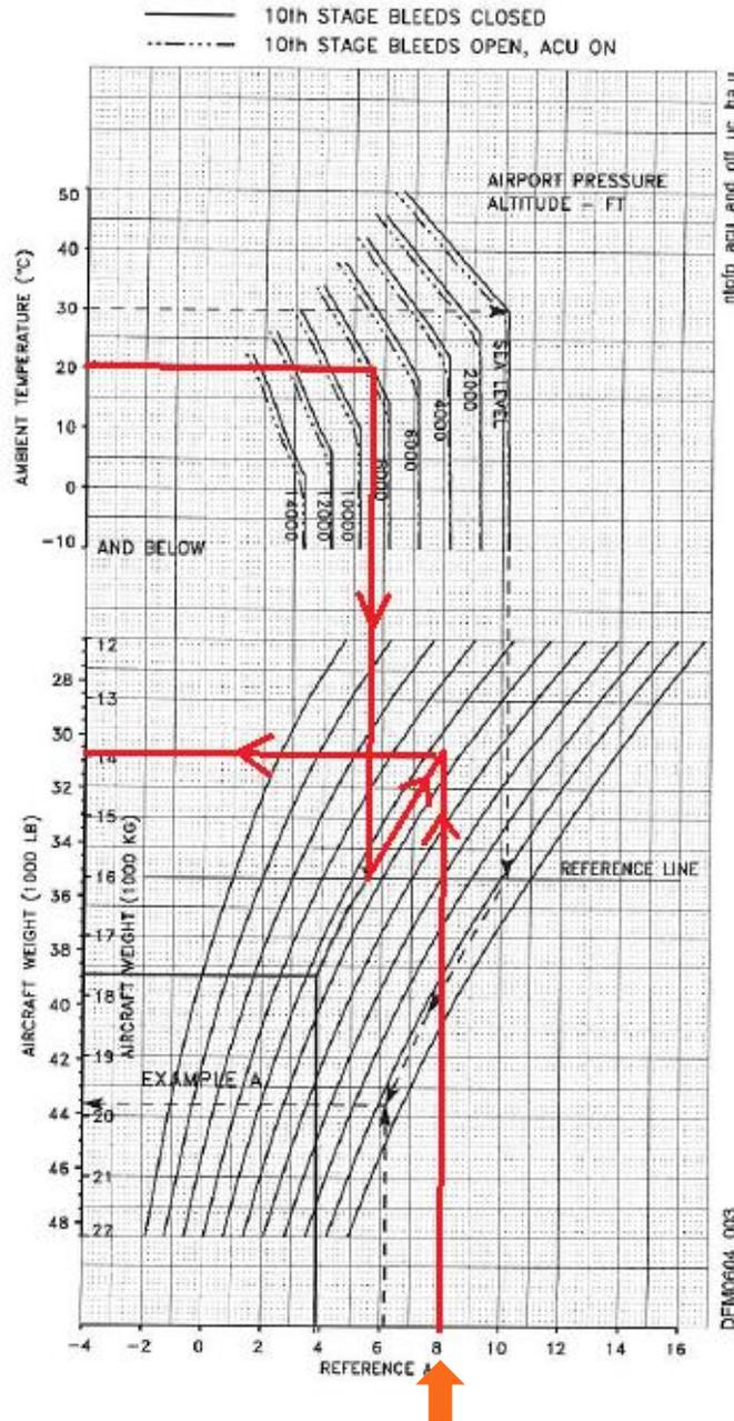
Obstacle Clearance Reference Climb Gradient, Flaps 20° - Anti-Icing Off (Page 1 of 2)
